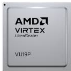
AMD/Xilinx Virtex UltraScale+ VU19P. 2020г.
